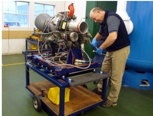
Arriel Engine Being Prepped for Test
