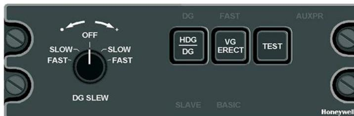
Typical AHRS Controller, photo courtesy of Honeywell International Inc.
